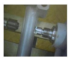
Finally, John demonstrated the Kiss Test to check that the lathe headstock and tailstock are correctly aligned. This involves a drive centre in the headstock and a pointed centre in the tailstock. These should meet point to point and remain so as the drive centre is rotated in the headstock. If they do not align then the position of the headstock must be adjusted.
